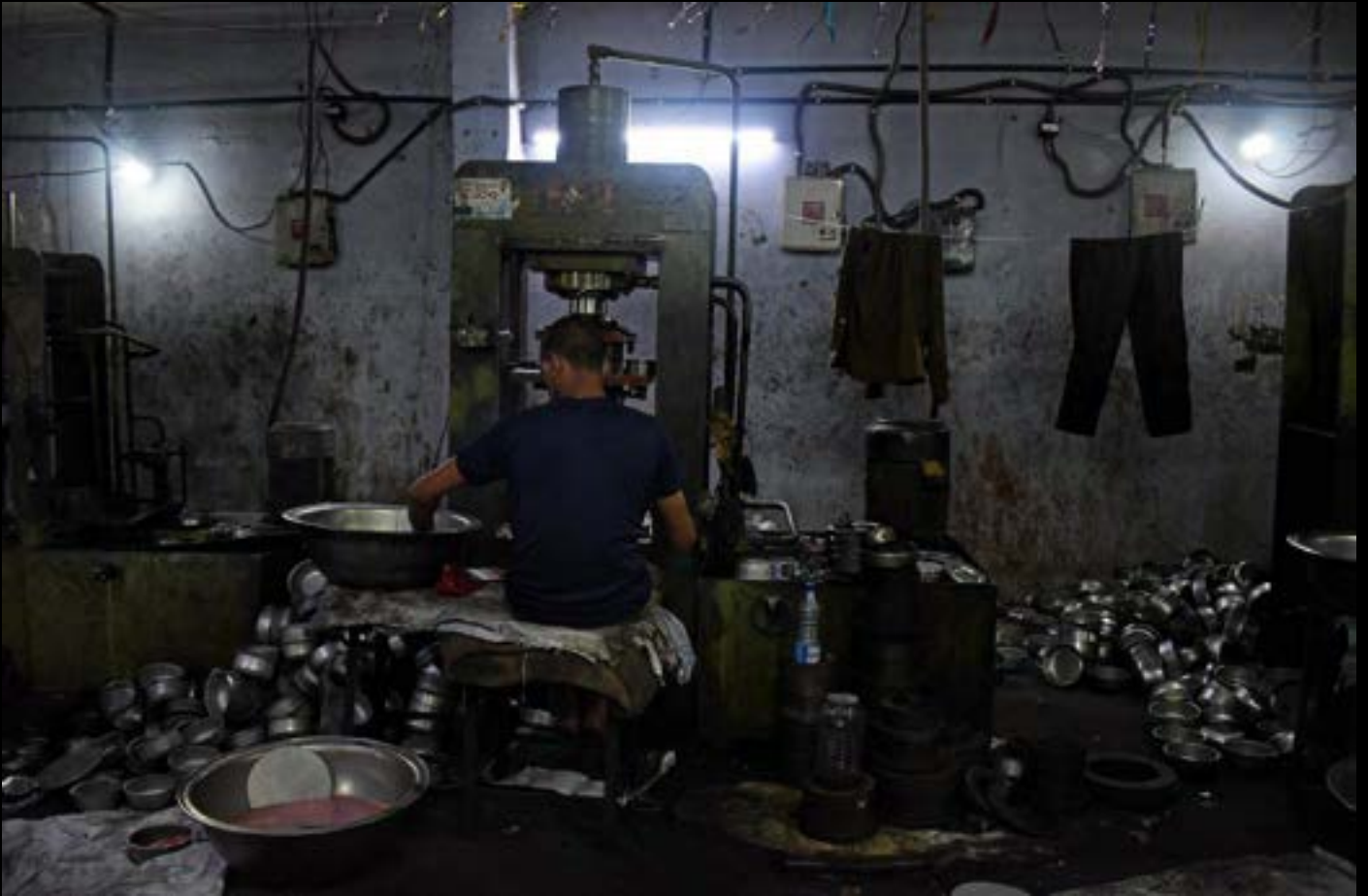
A Worker operates a power-press machine to shape steel containers
